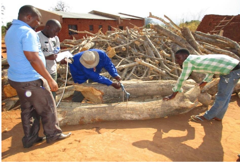
Figure 3.2: Caliper and linear tape being used to measure mid-diameter and length of the log
